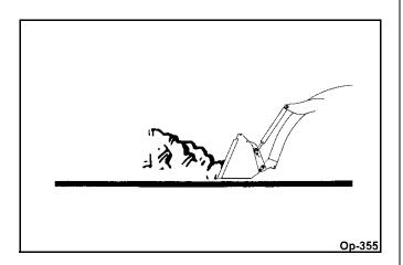
Loaders with 1-lever control, ease lever back toward you to lift and roll back bucket. With series valve, prevent loader stall by not lifting and rolling back at the same time.
